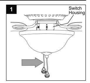
2. The pull chain located in the center is used to turn the *light* ON or OFF.
