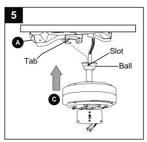
To ensure the safety of the installation and to prevent the motor assembly (C) from becoming or coming loose, use the plastic lock tab (L). Slide plastic lock tab (L) under bracket tabs so that it will snap into place.
